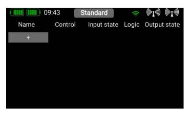
Select the **Virtual Switch** button in the menu, then press + to set up a new virtual switch. You can rename the virtual **switch** by pressing the switch button. As you can see, this field includes a small triangle at top right. This means that a function can be selected here by holding your finger on it. In this case the virtual switch can be erased again by holding your finger on the switch button.
