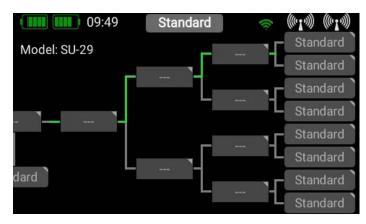
The most important thing to know at this point is that the **CORE** prioritizes the flight modes. Priority runs from left to right, i.e. the flight modes in the left-hand tree diagram have the highest priority, and those on the right the lowest priority. Even when the flight mode structure is complex, this means that you can, for example, overrule all other switch positions with a single switch, returning you very quickly to "normal" flight mode.
