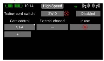
Repeat the procedure with the transmitter control from the Student transmitter: press the empty field under **External channel** and move the appropriate stick or switch at the Student transmitter. The **CORE** automatically detects which channel has been moved, and assigns this channel to the transmitter control at the **CORE**.
