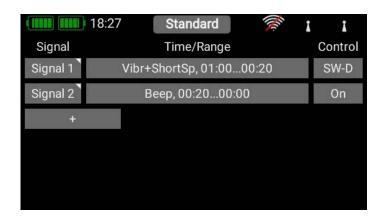
Press the \( \) button to leave Timer Setup. In the overview you will now see all the timers you have set up. The timer with the blue background is the one displayed in the current widget.
