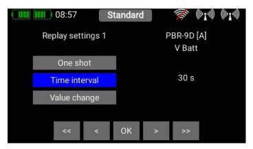
The **Once** option is used if you wish to have a timer or a telemetry value spoken when a switch is operated.
