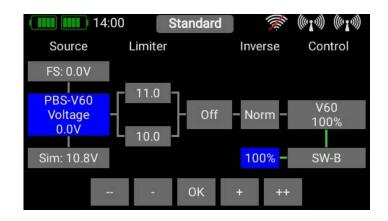
To conclude our example, you can now see how the telemetry control is set in such a way that motor power is reduced by 50% when battery voltage falls to 11.0V.
