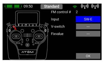
At this point you can select the appropriate transmitter control. If you select a switch, you can activate one or two switch positions. If you choose a linear control, you can set the switching threshold and hysteresis here. If you have already set up virtual switches, please note that you can also use these for selecting the flight mode.
