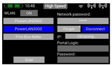
All passwords are stored in encoded form in the transmitter's Linux computer memory, and cannot be read out. The purpose of the Forget button is to erase this information.
