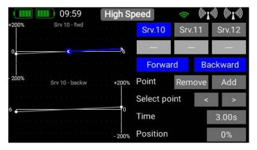
As you can see in the picture above right, an additional travel point has been added in the **Servo 10-Forward sequence**. You can now select the point you wish to alter using the arrow buttons after **Select point**.
