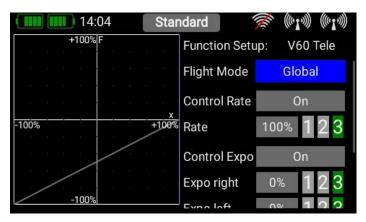
If the telemetry control is above the set value of 11.0V, 0% is added to the throttle servo, i.e. the throttle channel behaves in the usual way.
