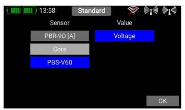
In this example the **PBS-V60** voltage sensor is to be used to reduce motor power if the voltage of the flight battery falls to a dangerous level. You can rename the telemetry control under the **Name** field.
