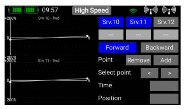
Below the **Srv.** buttons you will see two further buttons: **Forward** and **Reverse**. These buttons are also designed to display only those sequencer graphs which you wish to see or adjust at the moment.
