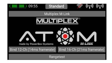
Choose your setting. If you do not need more than twelve channels, you should always give preference to **Option 12K**, as the servos are addressed at a higher rate in this mode. This can be advantageous in respect of smooth running, transit speed and precision. In contrast, **Option 16K** offers sixteen channels and a slower frame rate; this is the best choice for use with older servos.
