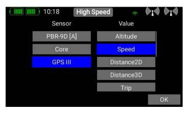
The left-hand column shows all the connected sensors, while the right-hand column shows all the values which these sensors supply. The **P**<sup>2</sup>**BUS** is an in-house development, and is capable of transmitting up to **255 sensors each with 32 individual values** – and at a speed of up to **800 values per second!**
