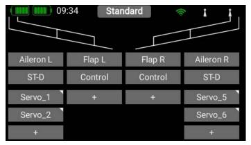
Briefly press Control, and move the aileron stick to select the Aileron control in the Context menu. Now you select a transmitter control which is to control the left aileron; this will be the left or right primary stick, depending on the transmitter mode you prefer.
